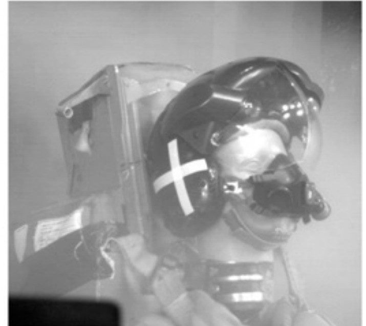
ABOVE The GENTEX MBU-20/P Oxygen Mask and the VSI Joint Strike Fighter (JSF) HMDS undergo successful windblast testing.
