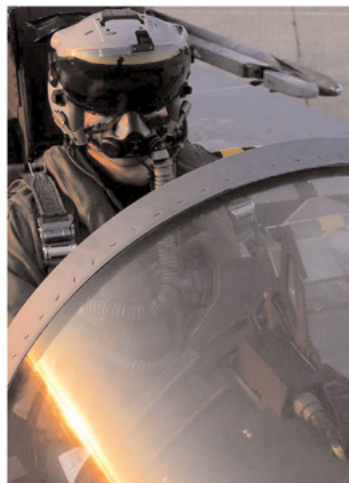
ABOVE VSI's JHMCS Integrated with GENTEX MBU-20/P Oxygen Mask, is currently in production and operational with U.S. fighter aircraft.
